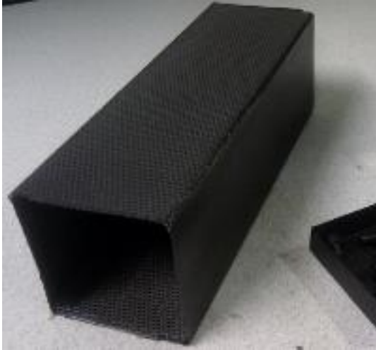
Fig. 9: Carbon Fibre prototype structure
