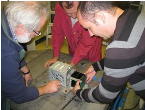
Fig. 4: Inserting HiNCube engineering model in the test pod for the vibration test.
